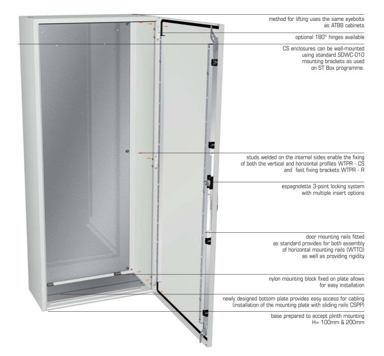
Ergonomic design and solid construction are the key features of the CS enclosure, providing the possibility to fit standard ETA system accessories as well as offering a large cable entry access for simple cable installation.
